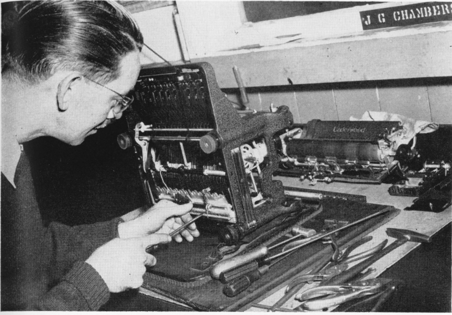
Here Johnny Chambers proceeds to dismantle a typewriter for repairs. Many needless repairs are the result of too-heavy beating on the keys, dropping the machine in transit, or failure to notify the repair man of odds and ends needing attention. Eraser crumbs cause lots of trouble.
