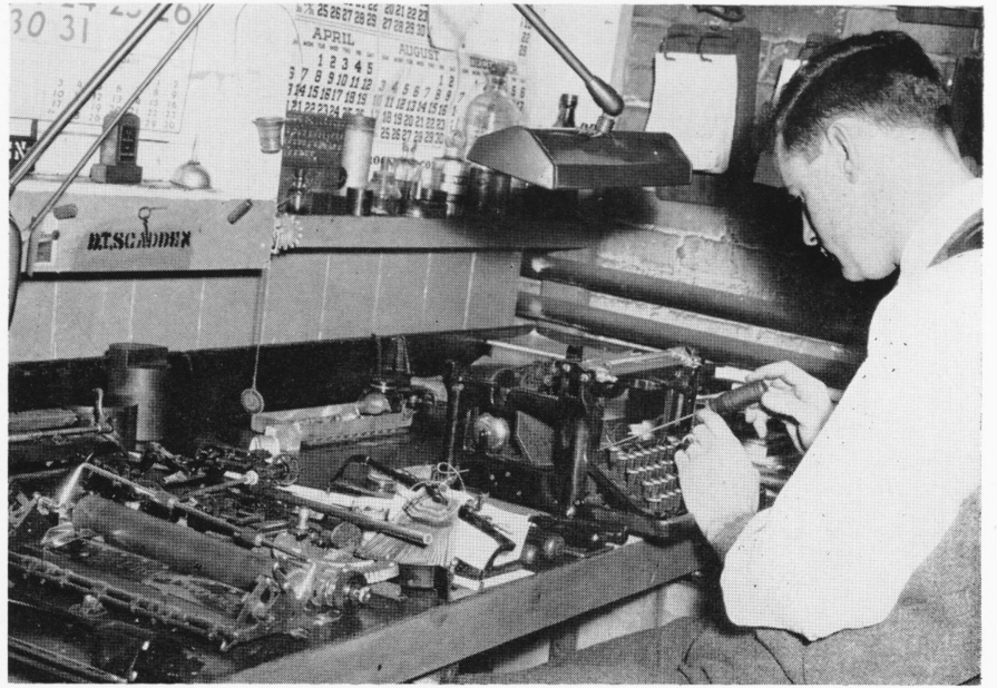
Dave has a machine in so many pieces as to mystify the layman. But he knows just where every part goes, having dismantled and put together thousands of machines in his time. This one is due for a complete overhaul job, new cylinder, ribbon, and rebuilt parts. The machine is returned completely spic and span.
