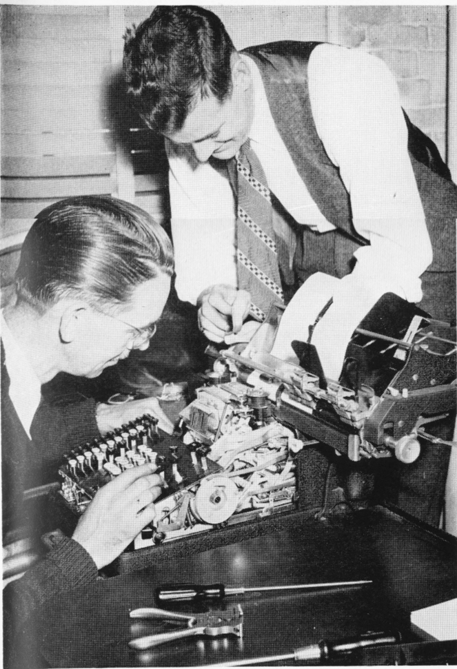
The posting machine in the Central Time Office is a complicated affair, and often two must do repair work on it at once. This is one of the machines used to record the payroll, and must never be off kilter.
